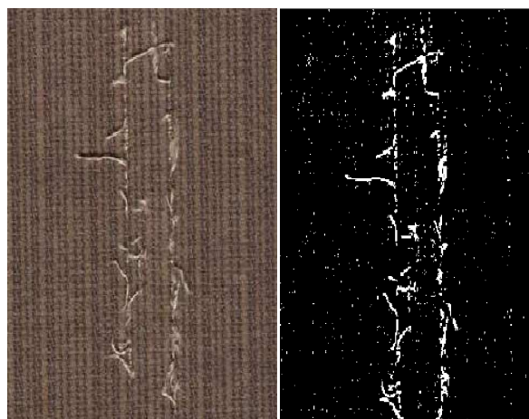
Figure 8 Detection of Scratch
